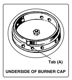
Be sure the burner cap fits correctly; the flame will not burn completely or correctly if cap is not positioned with Tab A in Notch B. **Keep the burner ports clear**. If the ports are clogged, use a wire, a straightened paper clip or a needle to clear the ports. **Do not use a toothpick; it could break off in the ports**.
